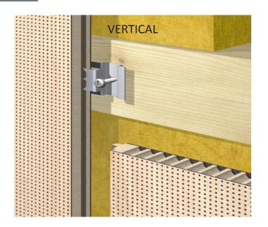
MOUNTED EITHER DIRECTLY TO A METAL OR WOODEN STUD, OR THROUGH DRYWALL INTO STUD OR BLOCKING, THE PLANKS ARE EASILY INSTALLED WITH A SIMPLE CONCLIP® FASTENER. PLANKS CAN BE INSTALLED VERTICALLY OR HORIZONTALLY ON BOTH WALLS AND CEILINGS.
